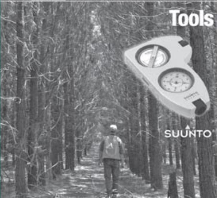
Combining a liquid damped precision compass and clinometer in one instrument, the Suunto® Tandem provides slope and height measurements as well as compass bearings. Designed for rugged field use, the Tandem's aluminum housing protects against impact, corrosion and water.
